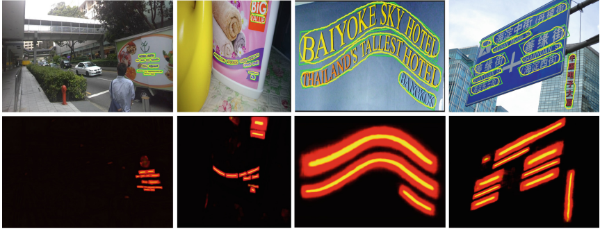
Fig. 8. Qualitative results by the proposed method. Top: detected text contours (in yellow ) and ground truth annotations (in green ). Bottom: combined score maps for TR (in red ) and TCL (in yellow ). From left to right in column: image from ICDAR 2015, TotalText, CTW1500 and MSRA-TD500. Best viewed in color. (Color figure online)
