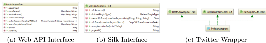
Fig. 3. The MINTE + framework defines three basic interfaces for a Wrapper: WebApi-Trait, SilkTransformationTrait, and OAuthTrait.
