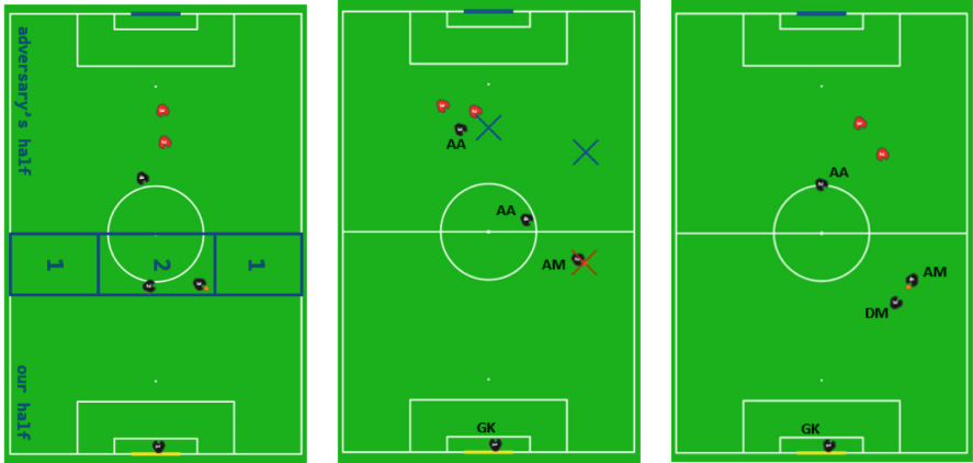
(a) For ball in zone 1, play 1 is executed, for ball in zone 2, play 2 is executed. For all other situations, regular game play is executed. Black robots: attackers, red robots: defenders. (b) Attack with STP: AM intercepts the ball (target red cross), AA's position in given zone (target blue cross). (c) Attack without STP: AM intercepts the ball, AA positioning on opponent half, DM positioning on own half.
