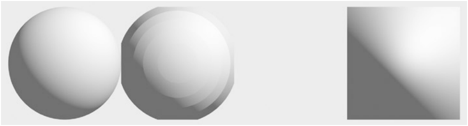
Figure 7-3. Four unit spheres ( r = 1 ) placed at distances of (from left to right) 100, 2000, 4100, and 8000 from an orthographic camera. Directly implementing Equation 3 can result in severe floating-point precision artifacts, up to missing intersections altogether, as for the 4100 case.
