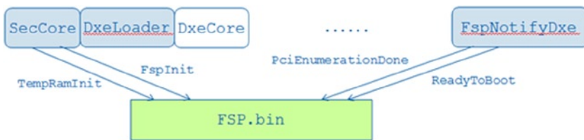
Figure 6-4. FSP wrapper boot flow option 1
