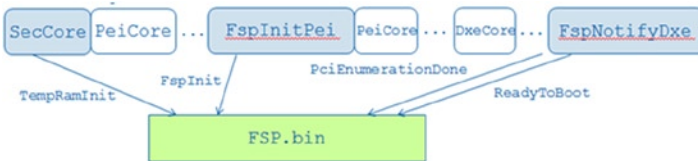
Figure 6-6. FSP wrapper boot flow option 3
