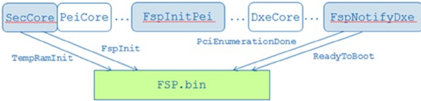
Figure 6-5. FSP wrapper boot flow option 2
