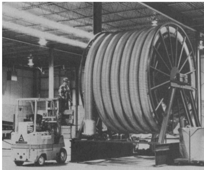
Fig. 21. Flexible gas-insulated transmission line under test at an EPRI facility. The development of flexible gas cable extends the advantage of SF 6 -insulated cable (low losses, inexpensive termination, and no oil handling equipment) to lower power levels (from 2000 MVA to 1000 MVA at 345 kV) and considerably improves the economics and ease of installation. It has been estimated that the flexible system will be about 25% less expensive on an installed basis as compared with the rigid-isolated phase gas cable. ( Electric Power Research Institute. )
