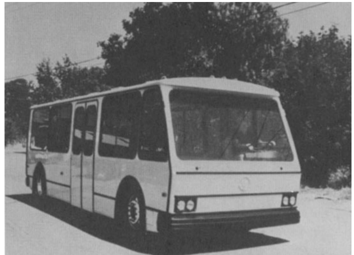
Fig. 3. The Electrified Roadway concept is scheduled for testing in a west coast city prior to 1990. Shown here is a prototype bus that will operate over a one-mile segment of electrified road. The propulsion battery is designed to be recharged as the bus travels over the electrified road segment. This will enable the bus to operate all day on both electrified and non-electrified segments of the proposed three-mile route. ( Electric Power Research Institute. )
