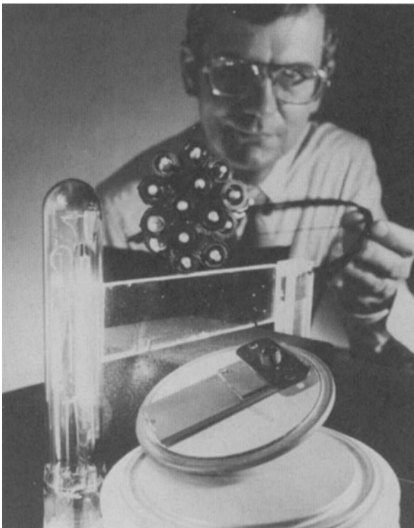
Fig. 14. In the late 1980s, electric utility industry researchers reported that increasing use of solid-state switching systems is being made in phase control and high-voltage dc converters. These systems are composed of a multitude of thyristor (silicon-controlled rectifier) switches connected in series/parallel configurations to provide high-voltage, high-current capabilities. Recently, it has become feasible to trigger high-power thyristor switches by the direct action of infrared (IR) light on a photothyristor. Systems using such thyristors have the advantage that the triggering light signal is carried by electrically insulated fiber optics, and special insulation is not required for the gate circuit. An additional advantage is that the fiber-optic cable is immune to electrical noise pickup and the attendant possibility of destructive accidental triggering. ( Electric Power Research Institute. )
