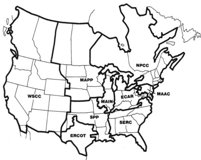
Fig. 6. Regional reliability councils that make up the total NERC network. Legend: ECAR (East Central Area Reliability Coordination Agreement); ERCOT (Electric Reliability Council of Texas); MAAC (Mid-Atlantic Area Council); MAIN (Mid-America Interpool Network); MAPP (Mid-continent Area Power Pool); NPCC (Northeast Power Coordinating Council); SERC (Southeastern Electric Reliability Council); SPP (Southwest Power Pool); and WSCC (Western Systems Coordinating Council). Also, not shown, is an affiliate, ASCC (Alaska Systems Coordinating Council).
