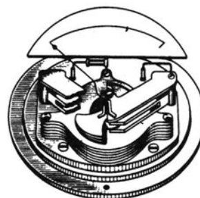
Fig. 11. Moving-and-fixed plate-type electrostatic instrument.
