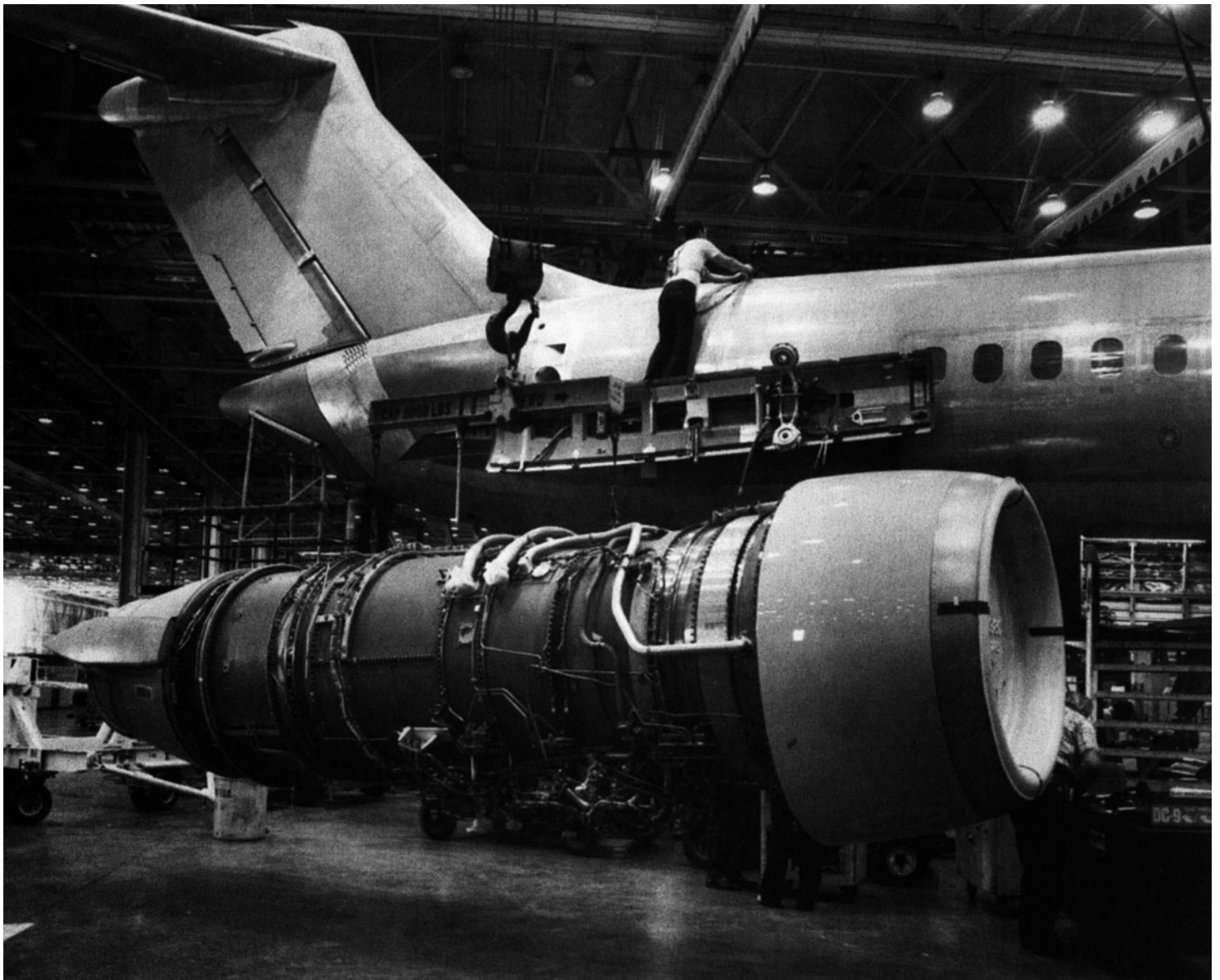
Fig. 3. Partially assembled DC-10 Series 30 aircraft (at height of production run in early 1980s), showing one of the three large jet engines in foreground being readied for attachment to the aircraft. (McDonnell Douglas Corporation.)
