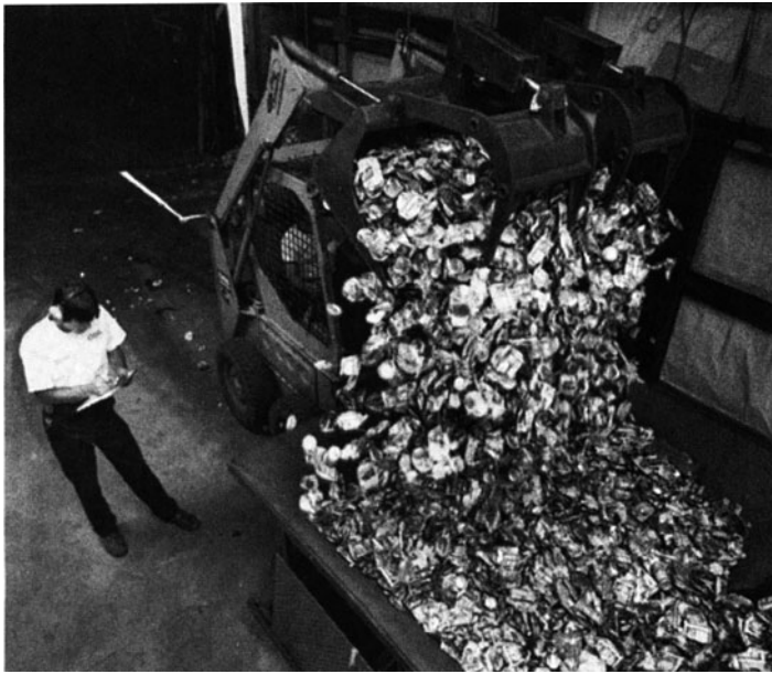
Fig. 2. Recycling of aluminum beverage cans and other scrap saves nearly 95% of the energy required when producing the virgin metal from ore. Approximately 50% of the metal processed in 1990 was recycled from scrap. (Reynolds Aluminum Recycling Company.)
