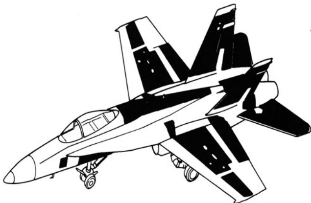
Fig. 16. Airframe of the F/A-18 strike fighter aircraft is a balance of conventional materials and graphite epoxy providing an optimum lightweight structure. The wing skins, trailing edge flaps, stabilizers, vertical tails and rudder, speed-brake, and many access doors are made of graphite composite materials comprising about 9.9% of the aircraft structural weight and resulting in appreciable weight savings, plus increased aircraft performance. Other materials used (as a percent of structural weight) include aluminum, 49.6%; steel, 16.7%; titanium, 12.9%; other materials, 10.9%. (McDonnell Douglas Corporation.)
