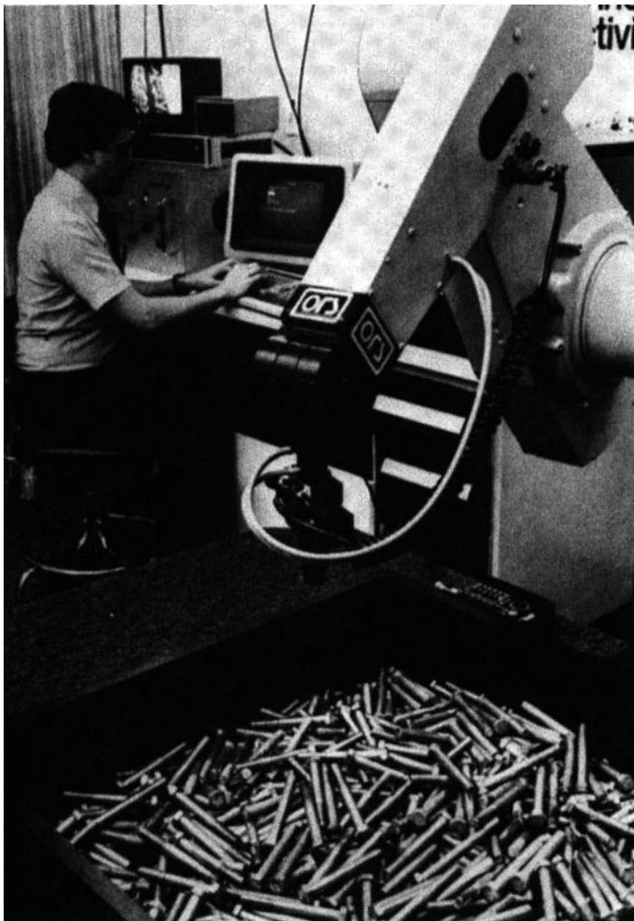
Fig. 1. Robotic system incorporating both machine vision and end-effector pressure sensors is designed for unloading randomly positioned parts from a storage bin. ( ORS-i-bot™ , ORS Automation, Inc.)
