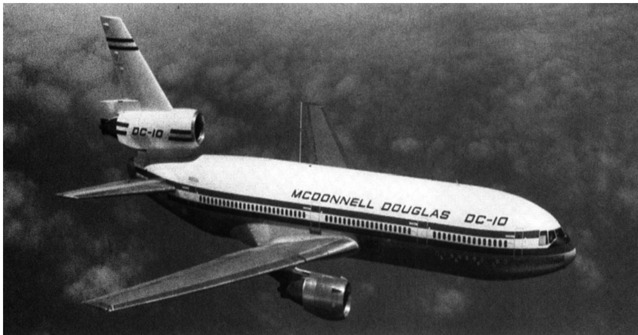
Fig. 1. The DC-10 ushered in the aircraft design era of the 1970s. For nearly 25 years, this has been a virtual workhorse of passenger aviation. The first commercial flight took place in August 1970. The DC-10, with many still in use, is powered by three engines ranging in thrust from 40,000 to 53,000 pounds (178 to 236 kN).
