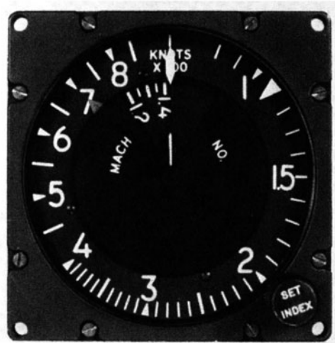
Fig. 4. Combined true-airspeed and Mach number computer indicator.
