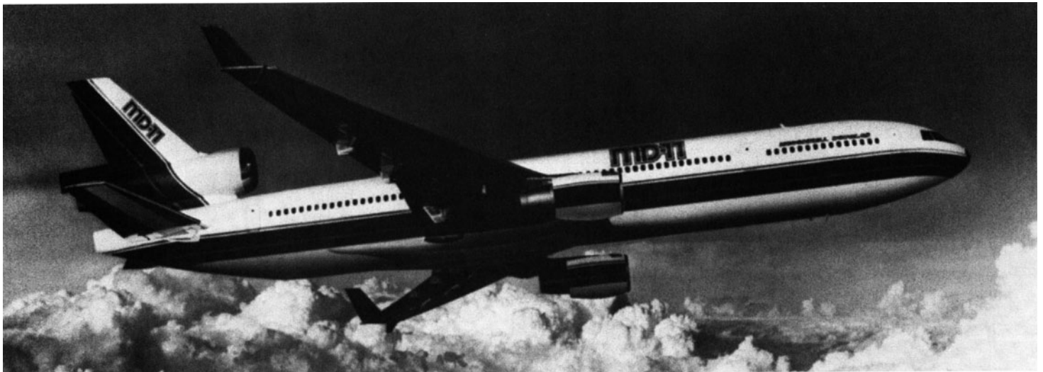
Fig. 5. The MD-11 tri-jet. The design is based upon experience gained from over 25 years of improving the DC-10. The MD-11 features a smaller horizontal tail and winglets (vertical airfoils at the wing tips). Both of these features contribute to improved range by reducing in-flight aerodynamic drag. (McDonnell Douglas Corporation.)
