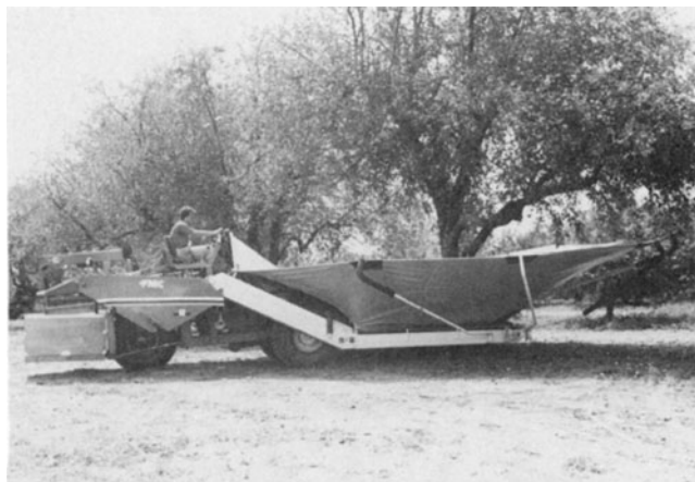
Fig. 12. Operator lining up mechanical shaking and catching machine in fruit orchard. A machine of this type can be used on apples, cherries, peaches, and various nuts. This machine was developed in the late-1970s. (FMC Corporation)
