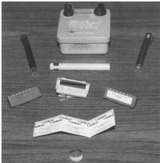
FIGURE 13.4 Individual dosimeters. These are some of the devices used to measure the exposure dose received by a worker. Front, ring dosimeter; second row, dosimeter film; third row, film badge holders—empty, open, and loaded with film; back row, pocket dosimeter and charger/reader.
