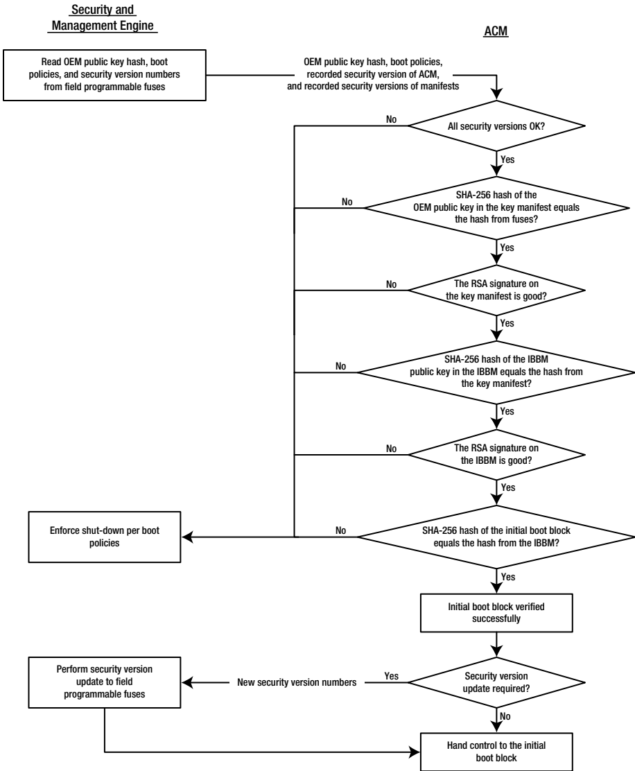
Figure 6-5. The initial boot block verification flow for the verified boot
