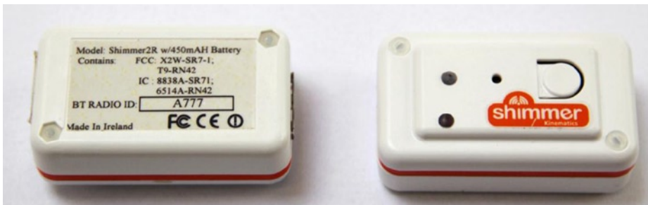
Figure 6-1. CE marking on a Shimmer device (reproduced with permission from Realtime Technologies Ltd)
