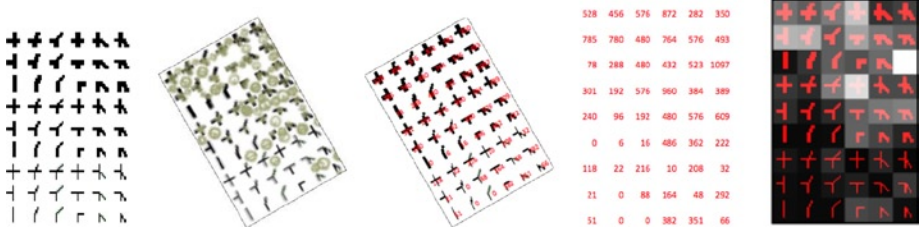
Figure A-26. Method of computing and binning detected alphabet features across rotated image sets, mocked-up SIFT data for illustration. (Left) Original image. (Center left) Rotated image annotated with detected points. (Center) Count of all detected points across entire image superimposed on alphabet cell regions. (Center right) Summary bin counts of detected alphabet features in grid cells. (Right) 2D histogram rendering of bin counts as an image; each pixel value is the bin count. Brighter pixels in the image have a higher bin count, meaning that the alphabet cell has a higher detection count
