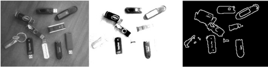
Figure 2-4. Use of thresholding to solve problems during image pre-processing to prepare images for polygon shape measurement: (Left) Original image. (Center) Thresholded red channel image. (Right) Perimeter tracing above a threshold
