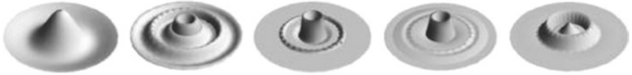
Figure 3-25. Various 2D wavelet shapes: (left to right) Top hat, Shannon, Dabechies, Smylet, Coiflett
