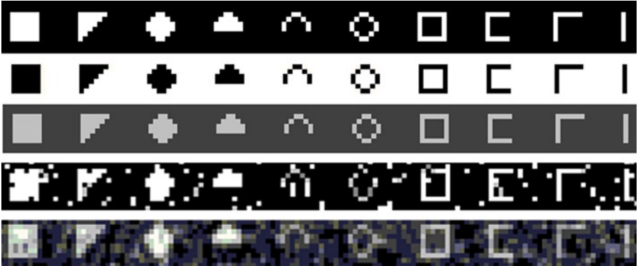
Figure 7-8. Portion of the synthetic interest point alphabet: points, edges, edges, and contours. (Top to bottom) White on black, black on white, light gray on dark gray, added salt and pepper noise, added Gaussian noise
