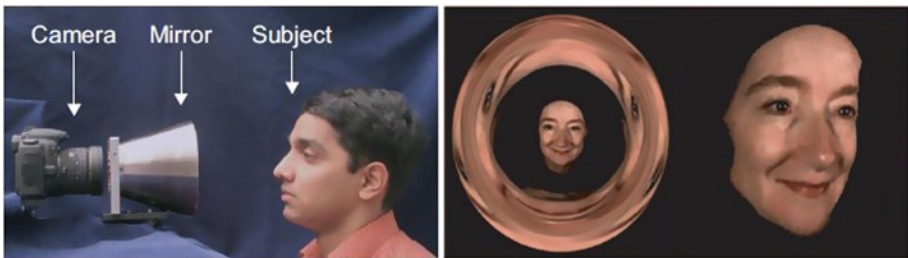
Figure 1-15. (Left) Radial camera system with conical mirror to capture 3D reflections. (Center) Captured 3D reflections around the edges and 2D information of the face in the center. (Right) 3D image reconstructed from the radial image 3D information and the 2D face as a texture map. (Images used by permission © Shree Nayar Columbia University CAVE)
