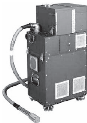
Figure 36.6. Example of fieldable pyMS based equipment: the CBMS Block II instrument.
