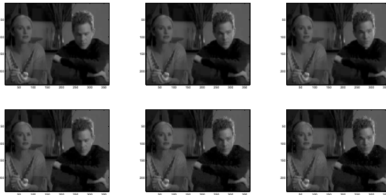
Fig. 7. Application level impact of our approach on high quality H.264 video comparing voltage scaled PCMOS [bottom](with an EPP ratio of 3.70X ) to the original H.264 frames [top]
