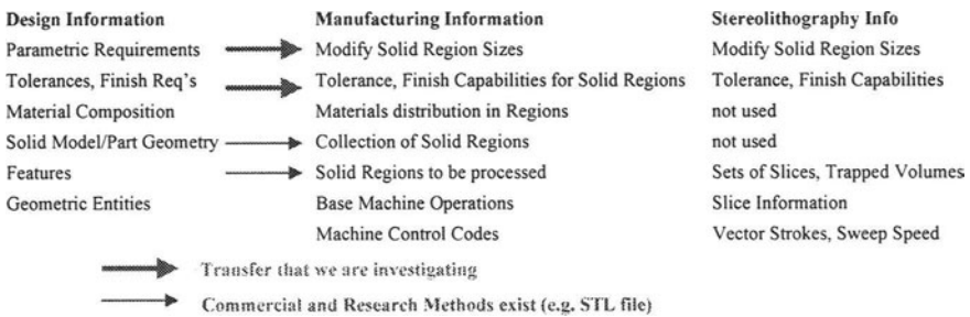
Figure 2. Information Hierarchies for Transferring Product Representations from Design to Manufacturing.
