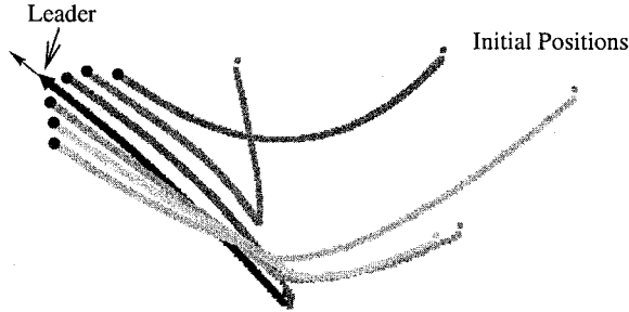
Fig. 3. Trace of the vehicles while forming and keeping a wedge shaped formation.
