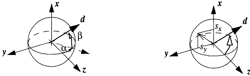
Figure 3. Euler angles parametrization (left) and axis-angle (right) of the swing motion.
