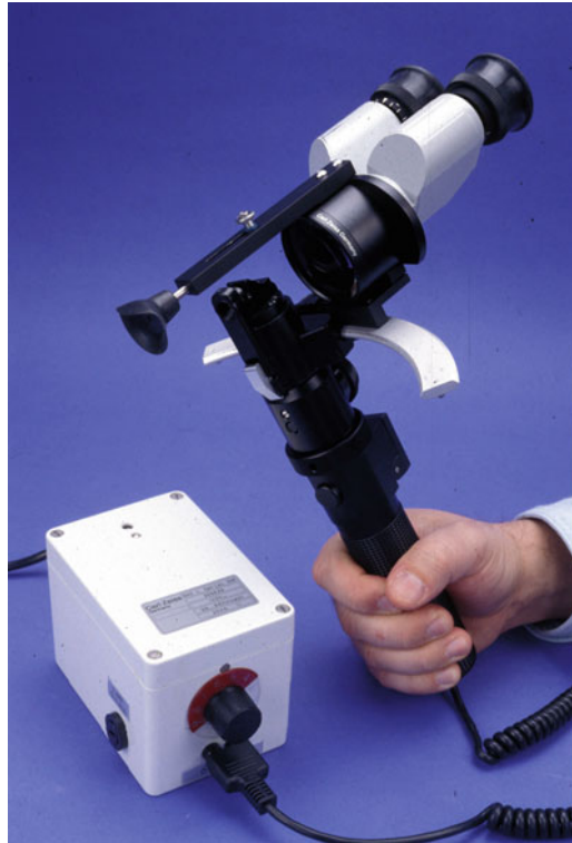
Fig. 1 A Zeiss HSO-10 slit lamp provides excellent optics and portability and is suited for use in all laboratory animal species
