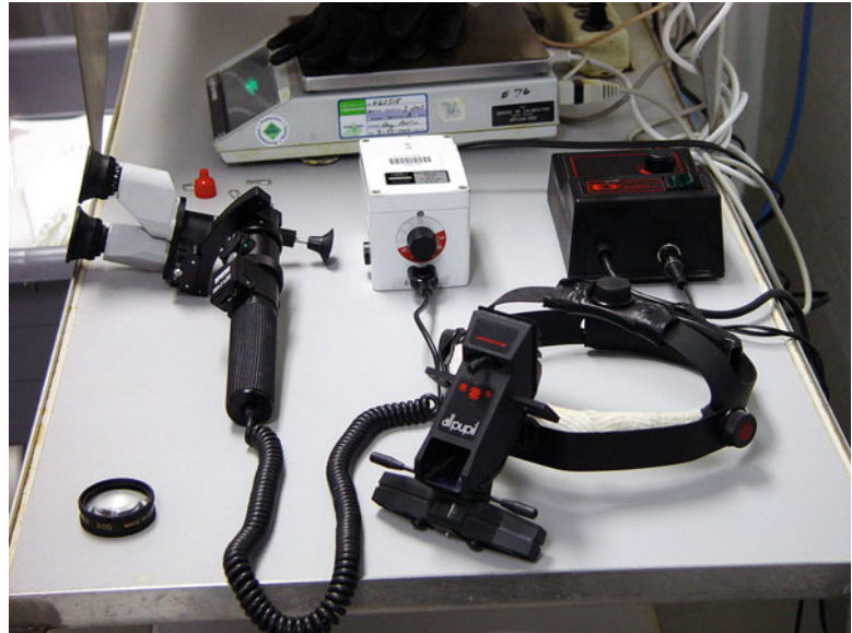
Fig. 11 A Keeler All-Pupil ® indirect ophthalmoscope, 30D condensing lens, and a Zeiss HSO-10 slit lamp used for ophthalmic examination of laboratory animals
