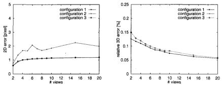
**Graphs 3 and 4: Behavior with respect to number of views.** The 2D error curves for the configurations 1 and 3 are nearly undistinguishable. The 3D error for configuration 2 lies above 5 %. The curve is thus not visible in the graph.
