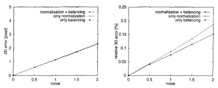
Graphs 5 and 6: Influence of normalization and balancing. The results presented here were obtained for configuration 1. The 2D error curve for "only balancing" goes off scale even for 0.5 pixels noise and the 3D curve is so steep that it is not even visible.
