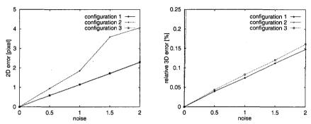
**Graphs 1 and 2: Sensitivity to noise.** The 2D error curves for the configurations 1 and 3 are nearly undistinguishable. 3D error for configuration 2 goes rapidly off scale.
