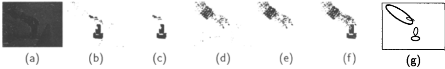
Fig. 2. The processing stages of our tracker. (a) shows an input image. (b) shows the coloured pixels. (c) shows the output of the region grower on (b). (d) shows the moving pixels. (e) shows the output of the region grower on (d). (f) shows the combination of (c) and (e). (g) shows the ellipses that are fit to the regions from (f).
