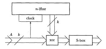
Fig. 1. A stage of the clock-controlled cascade
