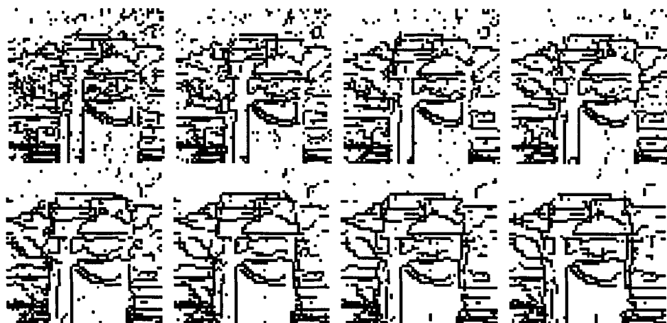
Fig. 6. Incremental Feature Extraction. The images show the evolution (left to right, top to bottom) of features over a ten image sequence.
