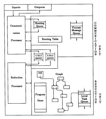
Figure 5: Structure of a Processing Unit
