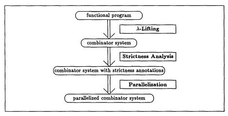
Figure 1: Structure of the Parallelizing Compiler
