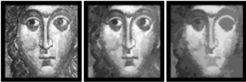
Fig. 3. An example of a pyramid of connected alternated sequential filters. Each contour is preserved or suppressed, but never deformed : the initial partition increases under the successive filters, which are strong and form a semi-group.
