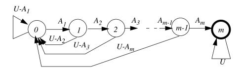
Fig. 3. A simple recognizer automaton, initial state is 0, state m is acceptin
