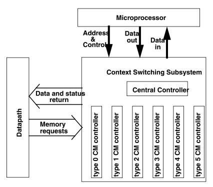
Fig. 1. Bock diagram of the Context Switch subsystem of FMD
