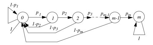
Fig. 4. Discrete time Markov chain for automaton in Figure 3
