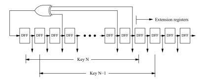
Fig. 7. LFSR with extension to save old keys.
