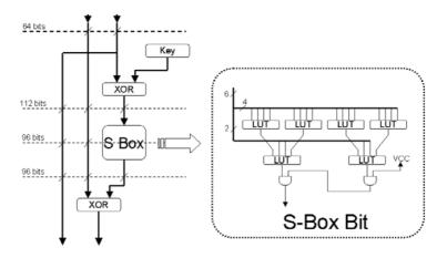
Fig. 8. S-Box details and pipelining options.
