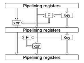
Fig. 6. Simple DES pipeline.
