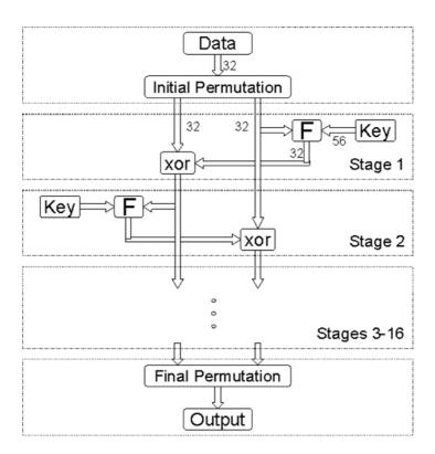
Fig. 1. The basic DES pipeline.
