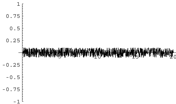
Fig. 2. Simulated correlation function g(t) between the points 4P_i and power consumption C_i(t) when d_{\ell-2} = 1 . No peak is observed since the points 4P_i are never computed by the card.
