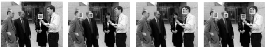
Fig. 6. Schematic illustration of merge from different channels. From left to right: Outputs of frontal, left, right view channels, and the final result after merge.
