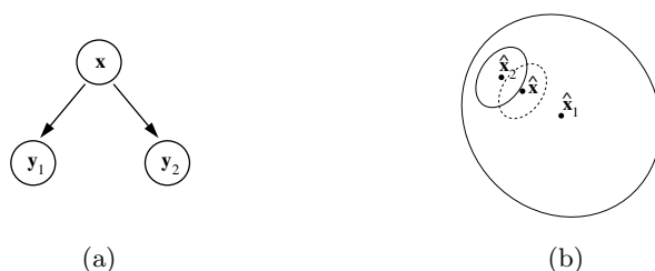
Fig. 2. The state of the world \mathbf{x} (a) determines the data sources \mathbf{y}_1 and \mathbf{y}_2 as described by this Bayes network, and (b) can be estimated as \hat{\mathbf{x}} by statistically combining the estimates \hat{\mathbf{x}}_1 and \hat{\mathbf{x}}_2 .
