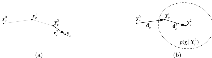
Fig. 5. (a) A model of errors in the partial results for cue c uses \mathbf{e}_c^i to represent the deviation in the partial result \mathbf{y}_c^i that will be eliminated by finishing the computation (which converges to \mathbf{y}_c ). (b) This model is a probability distribution on convergence location that is a function of the partial results seen so far ( \mathbf{Y}_c^i ).
