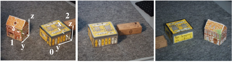
Fig. 3. Images and parallelepipeds used for calibration.
