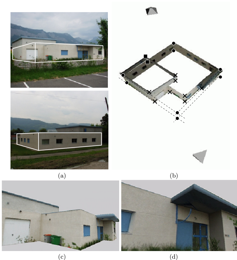
Fig. 5. Building reconstruction: (a) Original photos used for the reconstruction; (b) the reconstruction scenario with the computed model and camera positions; circles correspond to parallelepiped vertices, crosses and rectangles to points reconstructed from the first and second image respectively; (c),(d) Details of the model.
