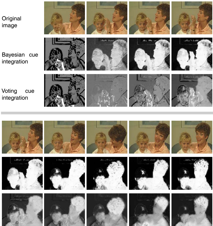
Fig. 3. Segmentation results from the “mother and daughter” MPEG-4 test sequence. The top rows show the original sequence whereas the middle and bottom rows show the belief of membership to the foreground for the Bayesian and voting integration schemes respectively. Bright areas indicate a higher degree of certainty. After the first few frames results improve as additional cues are trained and their reliabilities increase. Both integration schemes used self-organized weighting of cues according to general consensus.
