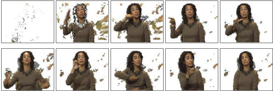
(c) The foreground person segmented out from the background. As before, results are poor in the first few frames before models are trained for cues other than motion.
