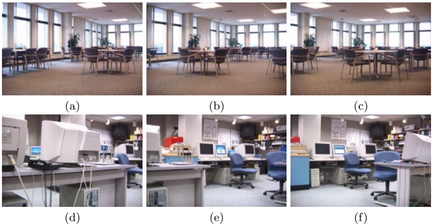
Fig. 4. Simulation results: a virtual bicentric image (a) is compared with the corresponding pinhole image as it would have looked without (b) and with (c) occluding surfaces. We also show two traditional panoramic images generated from roughly the same position as (a): (d) pushbroom, (e) cylindrical projection (panning, or self-rotating, camera).
