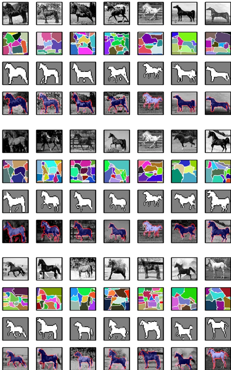
Fig. 10. Segmentation results arranged in 3 groups of 4 rows. First row in each group: input images. Second row: results obtained from low-level segmentation. Third row: class-based segmentation to figure and ground. Fourth row: segmentation superimposed on the input images (boundary in red).
