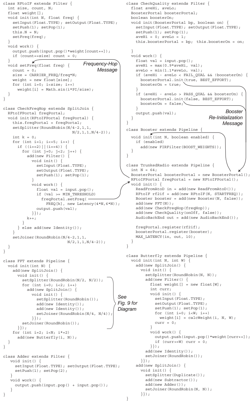
Fig. 8. StreamIt code for a software radio. Arrows denote the paths of messages
