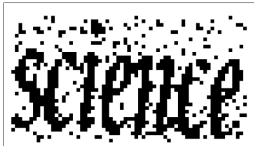
Fig. 5. Example of a PessimPrint challenge: an English word is chosen at random, then the word (as a whole) is typeset using a randomly chosen typeface, and finally the word-image is degraded according to randomly selected parameters (with certain ranges) of the image degradation model.
