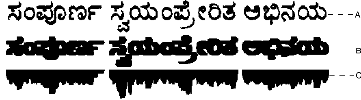
Fig. 3. Word segmentation: A. Input text line, B. Text line image after dilation. C. Vertical projection of image in B. The zero valleys in the projection separate the words.
