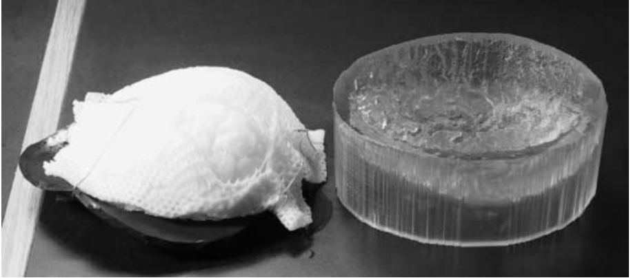
Fig. 2. The deformable PVA-cryogel phantom (left) and the mould (right) that was generated from a high-quality MRI scan of an actual brain.
