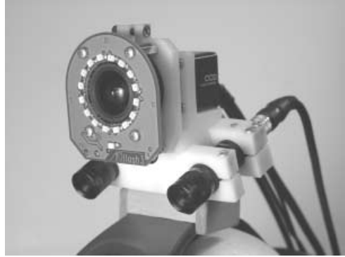
Fig. 2. Camera triplet with a stereo pair of camera to capture the scene and a dedicated tracking camera with infrared LED flash
