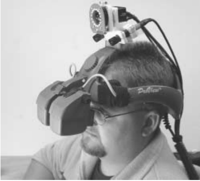
Fig. 1. Video-see-through HMD with mounted tracking camera
