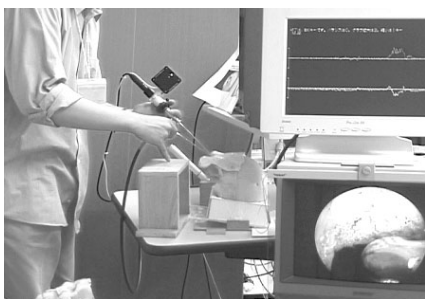
Fig. 1. Endoscopic sinus surgery training system. The endoscopic view ( lower right ) is also shown for the subject. The force output is shown on the computer display ( upper right ).
