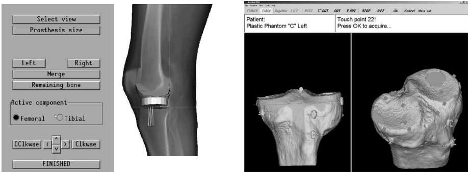
Figure 2. User interface of the planning software (left) and intra-operative user interface during anatomical registration (right)
