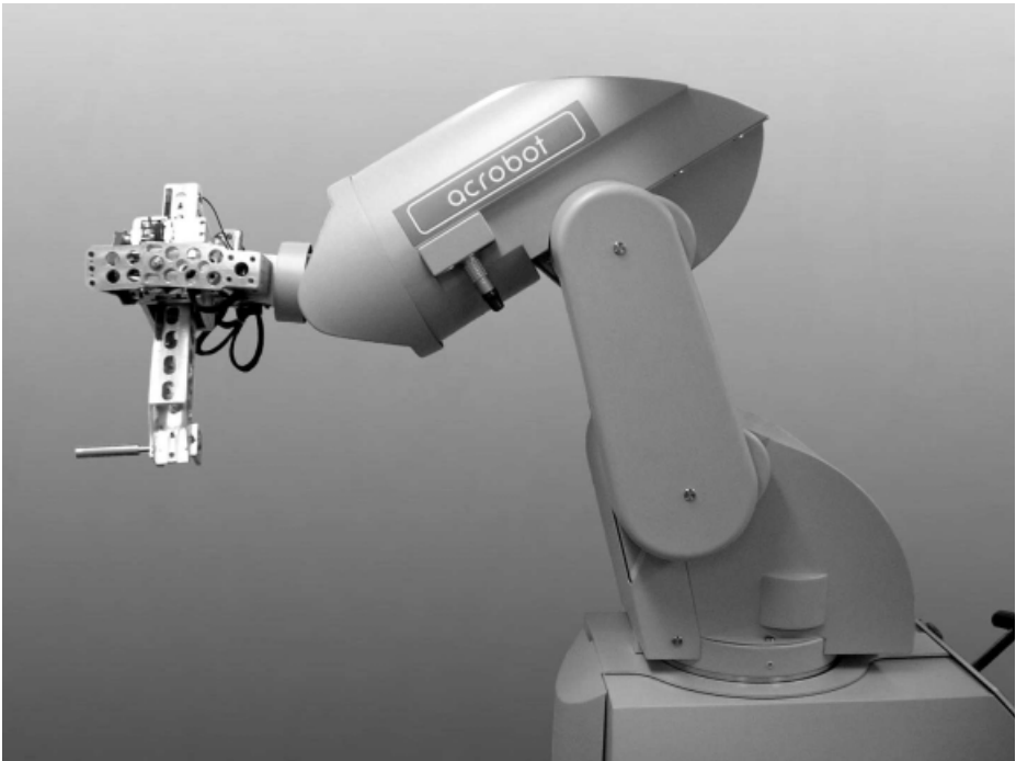
Figure 1. The Acrobot mounted on a gross positioning device
