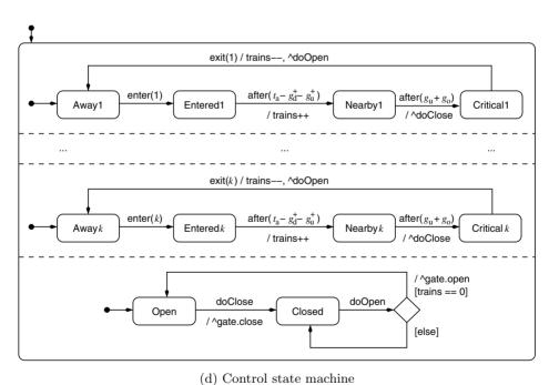
Fig. 2. UML model of the Generalized Railroad Crossing.
