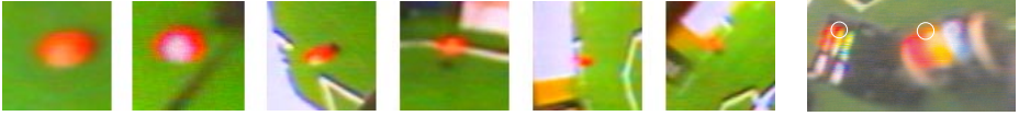
Fig. 3. The ball's appearance varies in color and shape and is similar to robot markers.
