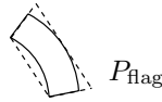
Fig. 1. Sector defined by an orientation and distance interval reconstructed by inverse quantization of raw server data representing the possible true relative positions of a landmark flag w.r.t. the agent. The solid line represents the form of the area as derived by the raw data. For the polygon algorithms, the area is slightly enlarged to the polygon denoted by the dashed lines.
