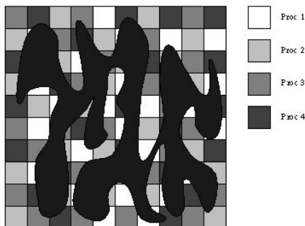
Fig. 4. Decomposition of an irregular shaped object in a 2D lattice. In this case 100 blocks are scattered over 4 processors.
