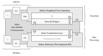
**Fig. 1.** The three conceptual layers of JULIUS, and the overall system architecture. Future developments can easily be integrated as modules or add-ins.
