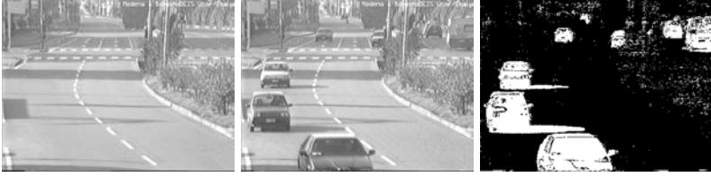
Fig. 2. The generated background (left), a sample frame (middle) and the thresholded background subtraction (right)
