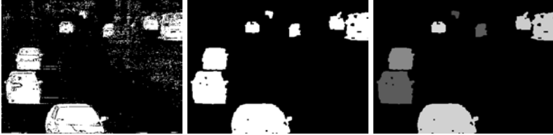
Fig. 3. The binary image after shadow removal (left), after morphological operations (middle) and the labelled image (right)
