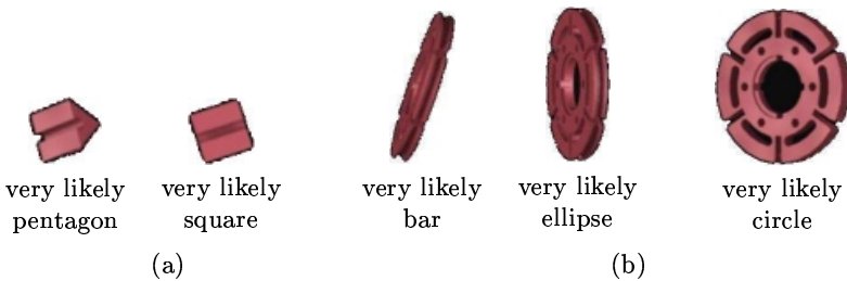
Fig. 5. (a) different views of the object 31010, one appearing as pentagon, the other one as square; (b) different views of object 31019 with the assigned symbolic shape descriptors
