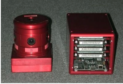
Fig. 1. Camera head (left) and storage unit (right) of Ladybug
