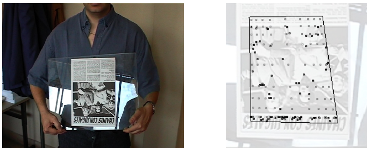
Fig. 3. Frame of a video sequence and its reference points. The quadrilateral represents J_0 . The interest points are in black, the regular ones are in grey.
