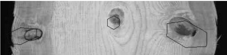
Fig. 2. Part of an optically scanned board with knots and detected knots overlaid
